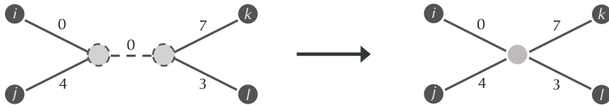
FIGURE 7.38 Gluing the nodes at the endpoints of an internal edge having zero length (shown by the dashed edge).
